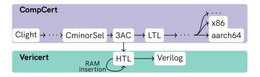
Current progress: fully verified HLS tool for a subset of C. Support for: all **control flow**, **fixedpoint**, **non-recursive functions** and **local arrays/structs/unions**.
